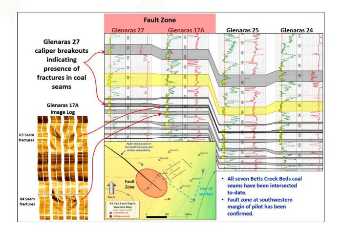
Figure 2 - Geological cross-section of Betts Creek Beds coals across the Pilot and the fault zone.
